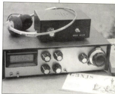
Home-brew QRP equipment can give great satisfaction when c.w. operating. This 3.5MHz transceiver has an additional digital frequency read-out and audio filter - the keyer on top is home-brew too!
